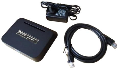
Site USB Device Server DSS-2 comes with a power adapter and an Ethernet cable.
