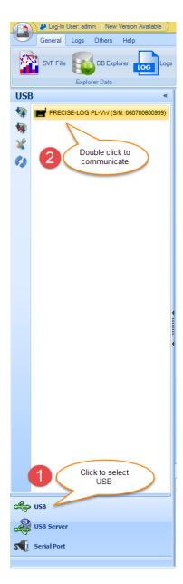
Double click on the icon to start the communication with the data logger. On the success of the communications, the status page of the logger will be displayed on the right side area.
